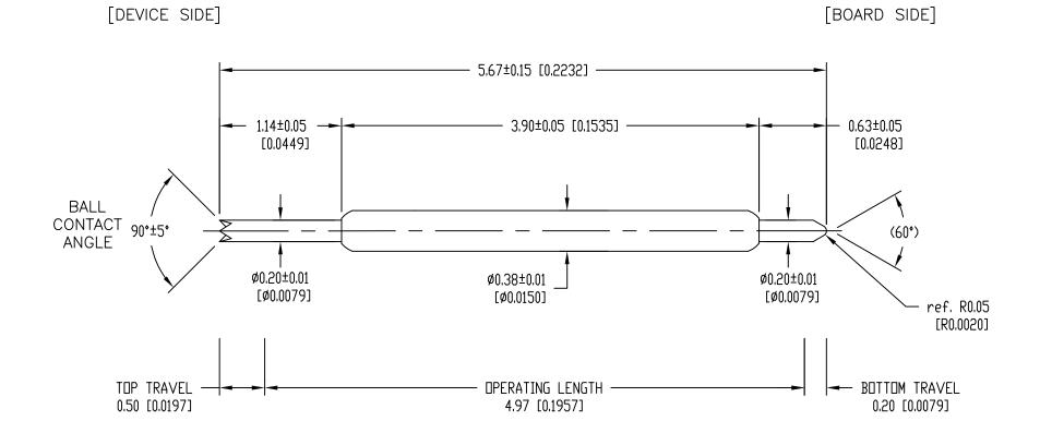
NOTICE: 0.20mm OR MORE OF PRELOAD AT BOTTOM SIDE IS A MUST FOR PIN DURABILITY WHEN SET IN DUT BOARD.
